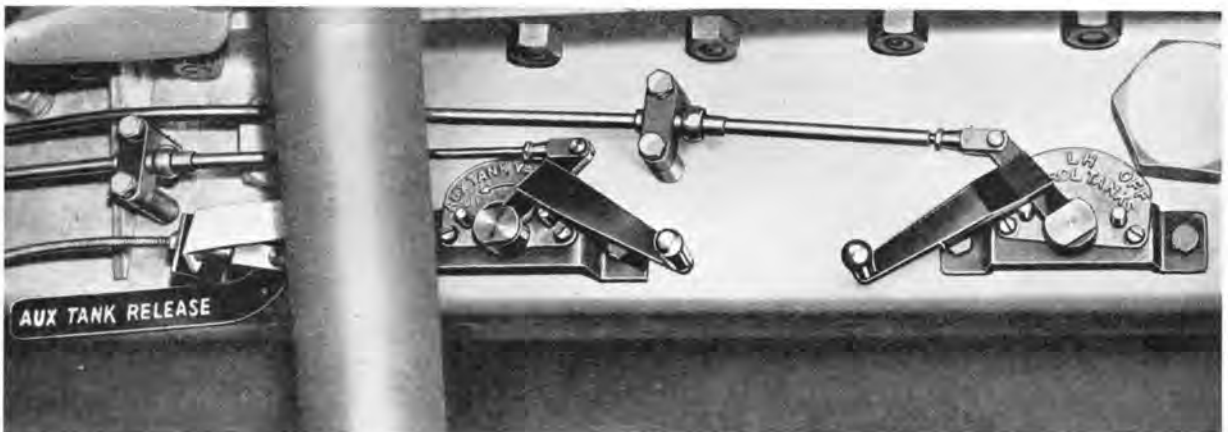
Fig. 12. Petrol tank controls. The auxiliary control is shown in the centre, the jettison lever on the left, and the main tank control lever on the right.
