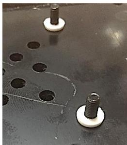
Fit the four screws through the bottom panel and place the insulators over the screw so they act like a 1mm space for the speaker. Fit the speaker and secure with the four M3 nuts provided. Attach two wires (about 150mm long) to the speaker and connect to the speaker out terminals on the PCB, connect the battery holder leads to the other terminals (make sure you connect this the correct way. )
