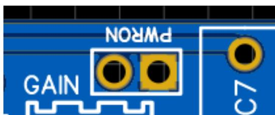
The Led is fitted just in front of the Gain control. You will see that there are two holes for it. One of the holes is square and the other is round. The LONG leg of the LED MUST go into the ROUND hole. Fit the LED so it stands with about 12mm of leg above the board.
