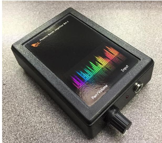
Fitted with a quality 2 inch one watt internal speaker and 6v battery pack (4 x AAA cells) its ready to be used when needed.
