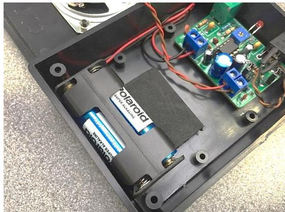
Fit 4 x AAA batteries into the holder and turn on the amplifier, the red LED should light up. You can test the amplifier at this stage but the audio quality will not be too good until the speaker is mounted inside a closed case. Now fix the speaker plate to the main body of the amplifier using the 4 small screws provided and then the stick on rubber feet. Carefully peel and fit the supplied sticker onto the top case (if not already done for you)
