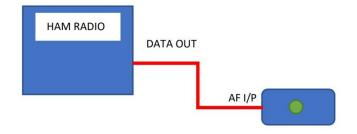
Plug the Magic Eye into a Data out / Tape out, or any Low level audio out from the radio. No mods needed to the Magic Eye
