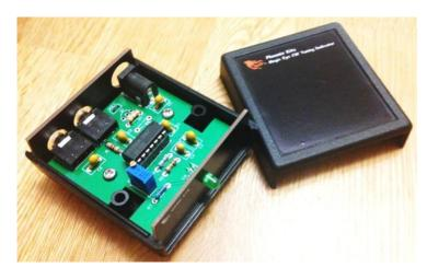
radio or plug into the external speaker circuit). The module will accept a wide range of input voltages from just a few mV up to several volts of audio.
