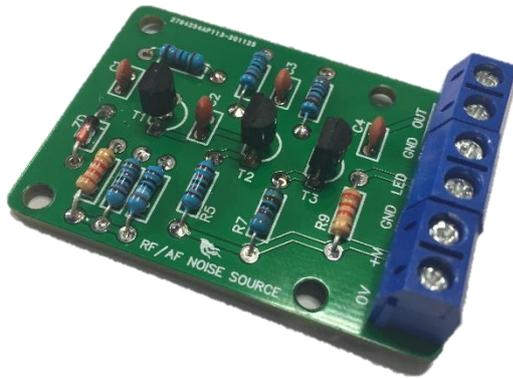
This Kit is designed to help with setting up Receivers filters and audio projects. It will produce strong white noise signals. Starting at audio frequencies right the way into the VHF spectrum. It is not a calibrated test instrument but uses the well know 'Noisy Diode' method of noise production that is amplified by 3 stages to produce a strong signal.
