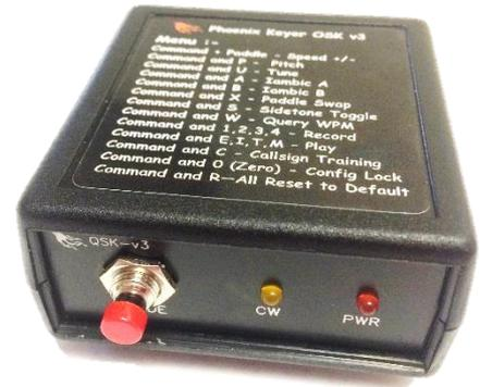
This open source code is now installed it onto an Attiny85 chip. The kit produces a desktop mounting Keyer with many options.
