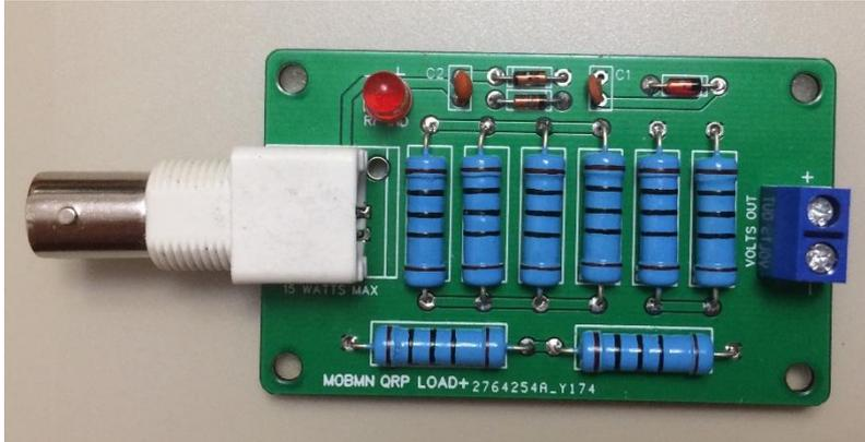
The QRPLoad+ is a QRP+ dummy load with a RF detector circuit that allows a standard Voltmeter to be used to measure RF power out, ideal for anyone adjusting homebrew QRP Transmitters. It also as an LED indicator to show when RF is present. Power as low as 50mW (or even lower) will cause the LED to light.
