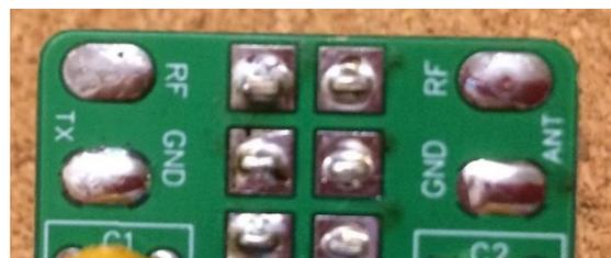
The board is marked TX (RF/GND) and ANT (RF /GND)
