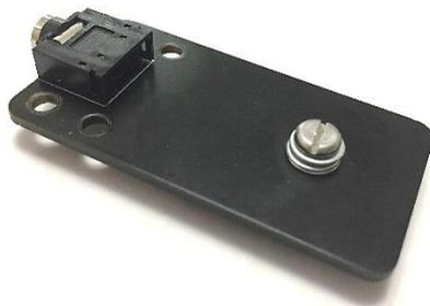
Now fit the bottom contact screw. Find the 6mm Screw (The shortest in the kit) and BEFORE putting it on the bottom board put three of the M3 Steel washers onto the screw. Put the screw through the single hole at the one end of the base panel away from the jack socket. The head of the screw needs to be on the same side as the jack socket. The screw head is the bottom key contact. This screw is then fasten to the board by putting a M3 steel nut under the board. Tighten the screw so it's secure.
