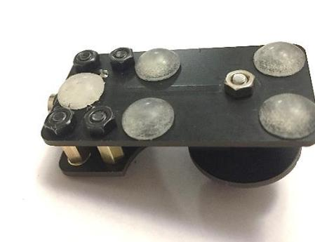
That's it the key is built and ready to test, connect a lead from the keys socket to the radio or oscillator and tap away.
