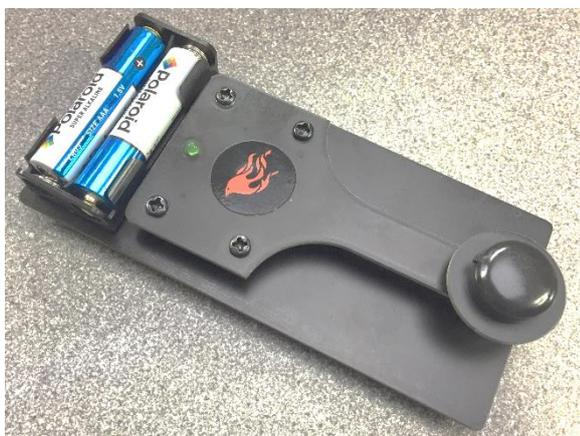
The sticker has not just be included for cosmetic reasons. Try this, hold the key down. Now place your finger tip over the hole in the top of the key panel, you will note that the tone changes. I feel it sounds better with the hole covered, the back pressure blocking the hole just above the sounder changes the pitch and tone qualities. If you agree then place the sticker over the hole.
