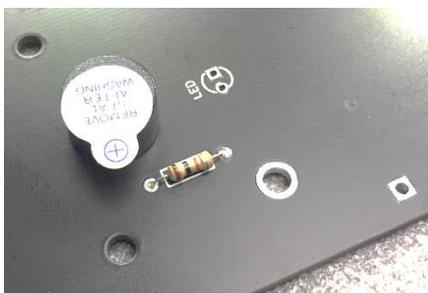
Next fit the 1K resistor. It is the only resistor in the kit, it can be fitted either way around.
