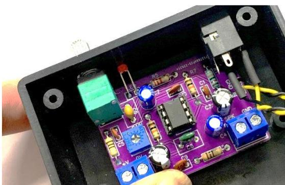
Carefully push the board forward so that the LED goes into the 3mm hole and the volume control goes into its hole, the LED will fold back on itself as it goes through the hole.
