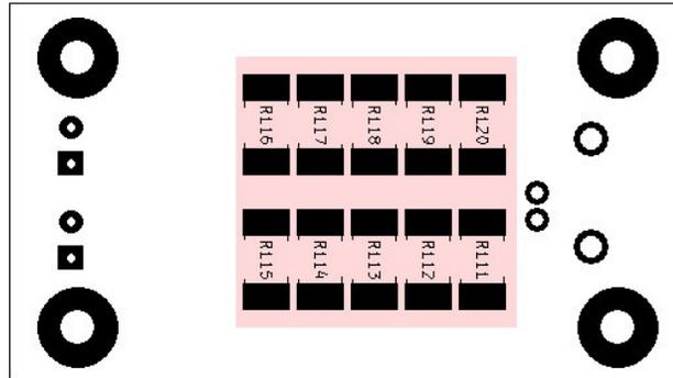
2. ( ) With an Ohm meter measure the resistance from the center pin of P101 to ground (one of the outer pins). There should be 100 Ohms of resistance when all 10 resistors are soldered. This completes the bottom side.
