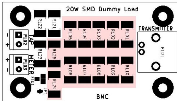
4. ( ) With an Ohm meter measure the resistance from the center pin of P101 to ground (one of the outer pins). There should now be 49-50 Ohms of resistance when all 20 resistors are soldered.
