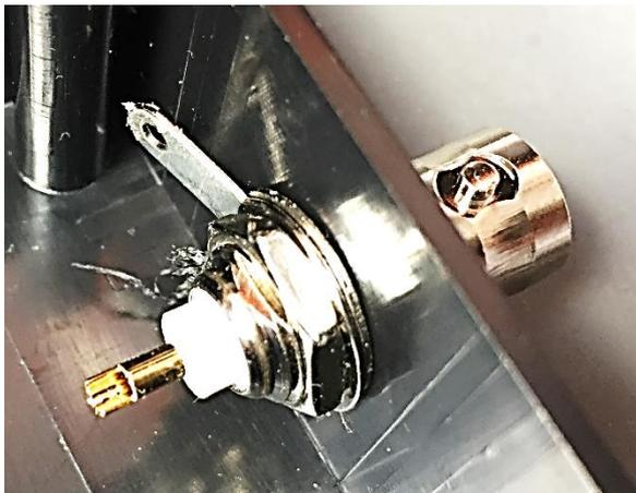
Now fit the BNC socket to the case, You may find it better if you can solder two 50mm wires to the socket (one to the centre pin , one to the tag) before you assembly it onto the case. Take care with this stage and don't hurt your fingers when tightening the BNC. Ideally use a BNC wrench to hold the BNC and stop it from turning while you tighten the rear nut, don't forget to fit the earth tag.
