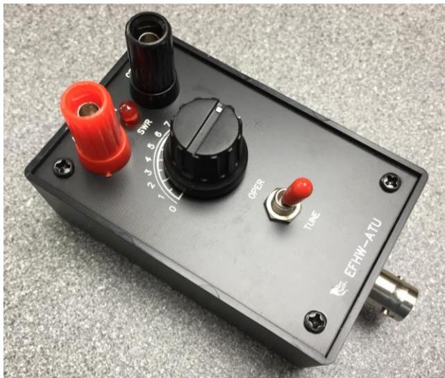
Turn the shaft of the capacitor towards the number 12 on the scale, now fit the supplied knob. The screw should be nearest the number 1 on the scale.
