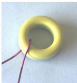
Start with passing the wire through the core as shown. Now wind 3 turns around the core, each time the wire passes through the core it counts as a turn. The short end of the wire should be down at 6 O'clock position as we start winding up towards in the 9 O'clock direction
