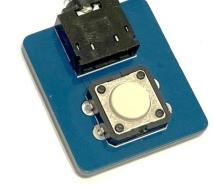
(12mm) tactile switches, one acts as the left paddle and one the right, there are two links that need to be made which allow the key to be set for left or right handed use (swaps the paddle sides around). To use the device, simply plug a standard 3.5mm lead into the jack socket of the key and the other end into your radio. These keys are very basic and have no adjustment but will get the job done when all else fails.
