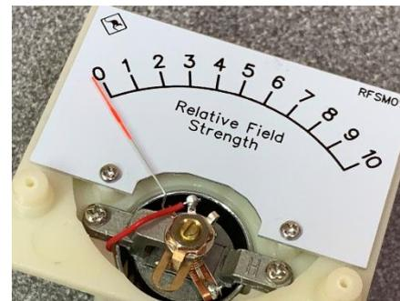
Now remove the meter scale screws (don't mix them up with the lid screws) , CAREFULLY slide the meter scale off the meter and replace it with the Custom new meter scale, secure with the two screws you removed a moment ago. Now refit the top lid to the meter.
