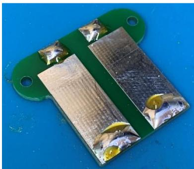
Apply a generous amount of solder to the two small square pads, don't worry about the small holes in the centre of these pads, we are not going to use them. Also apply solder to the bottom of the large rectangles as shown in the picture to the left.
