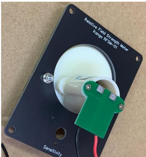
Next we need to fit the small FSM PCB and Pot to this panel.
