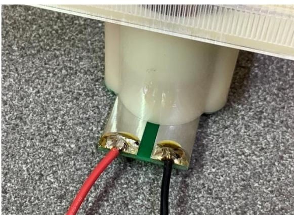
Now the last part of this stage is to attach the two meter leads to the termination PCB. You will have already put solder 'blob' on the bottom of the two rectangles. Use the supplied Red and Black 50mm wires for this. The wires are not the normal PVC type that shrinks when you solder them, there are high quality silicon coated wires and are very flexible.
