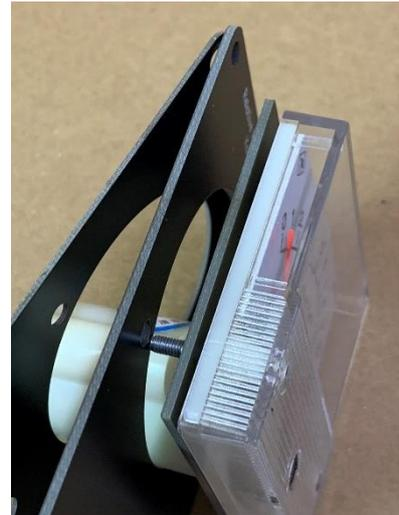
Secure the meter to the plates.
