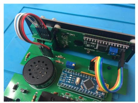
If you wish you can now test the tutor, to do so we need to fit the cables between the board and the front panel. The first is for the display, take the 4 way cable that came in the kit and plug it onto the main PCB.
