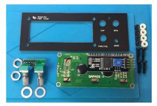
Fit the LCD module as shown below. Make sure that you put the small white spacers between the panel and the LCD display or the display will not sit correctly.
