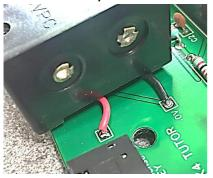
Then position the holder so the wires are under it and secure in place from the BOTTOM of the board with the three small black selftappers provided.
