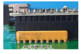
Note R3 is a bank of network resistors and must be fitted the correct way round.
