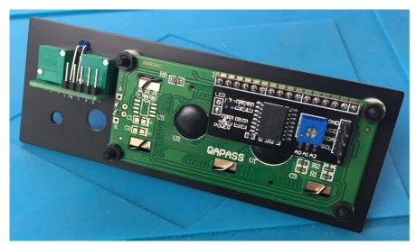
Note the pins on the display module in this picture. They are sticking out straight. Your module will have pins bent over by 90 degrees. You will need to straighten these pins. Use a pair of pliers and carefully bend the pins back to the upright position. Make sure they are nice and straight and all the same distance apart.
