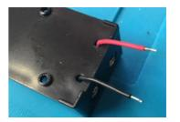
mm and twist/ tin the ends, solder the wires in place
