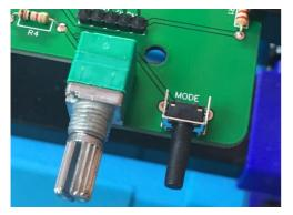
Now fit the mode switch, this fits next to the volume control on the PCB.
