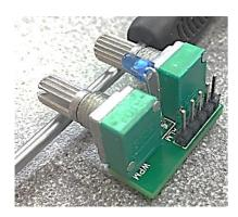
Fix the two 10K control potentiometers on the board, then the blue LED, the led should be fitted so it is a high as possible, just make sure the pins go through the board and no more. The LED as two leads, one longer than the other, the long pin goes into the ROUND pads hole.
