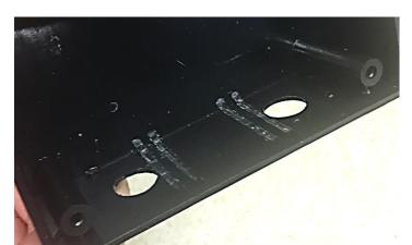
If these guides are not trimmed flush the BNC sockets will not mount correctly. A sharp pair of flush cut wire trimmers do the job quickly and easily.
