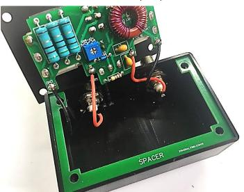
the box, the solution turned out simple. I used some 1.5mm thick washers to start with, it worked but it was hard to keep them in place while fitting the front to the case. In the end I had a spacer made that drops in between the front panel and the case. Make sure you drop this in before tightening the front panel down.
