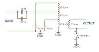
The number of turns on the output stage could be adjusted to work with lower impedance antennas ( try just 3 or 4 turns if you want to play) the only problem with reconfiguring this setup is that efficiency can suffer
