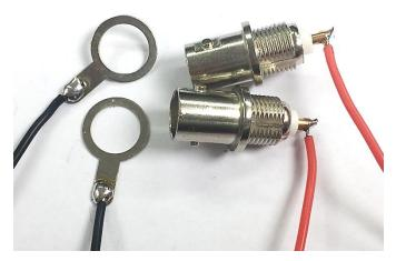
First solder the supplied wires to the BNC's and their earth tags. Now this is a tight fit in the case so solder the center pin of the BNC socket so the wire comes off at 90 degrees to the brass pin (see Photos). This is important or the wires will stop the board fitting into the case properly.
