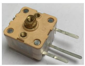
If you have a suitable capacitance meter check between the center pin and the two outer pins, you should find that you have about 250-270pf when you adjust the capacitor between each pin and center.
