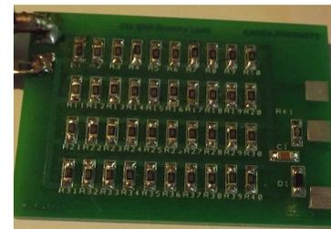
A dummy load is a resistor equal to the output impedance of a transmitter. It is used to convert the output power to heat instead of feeding it to the antenna.
