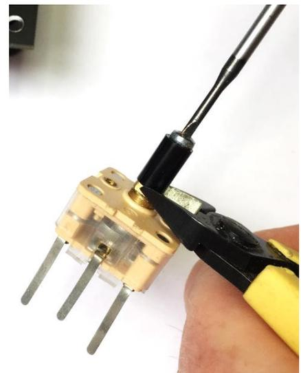
On the back of the capacitor you will see two adjustable trimmers set these to be fully open. Make sure you fit it the way shown here, you will be provided with two short flat head steel screws to fit the capacitor to the front panel.
