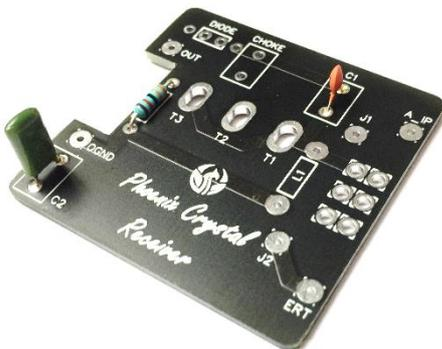
The PCB is designed to make building the crystal radio very easy and trouble free. Larger wide spaced pad have been used so it's suitable for beginners to build (With care!).
