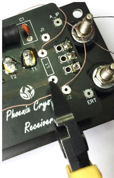
The two white wires need to be trimmed and soldered to the position marked 'L1' on the board, these wires have a very thin insulation on them that will burn off when you solder them in place.
