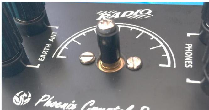
Fit the tuning knob. I just tighten the knob a little at first, just so it grips very slightly, then turn the tuning control and set it so it points correctly. Once you have it set correctly set the control to point upwards and then you can get easy access to the fixing screw, tight then screw to secure the knob.
