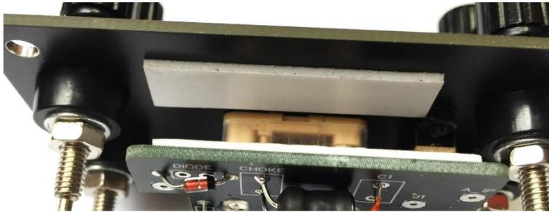
These foam strips help hold the coil in place later.
