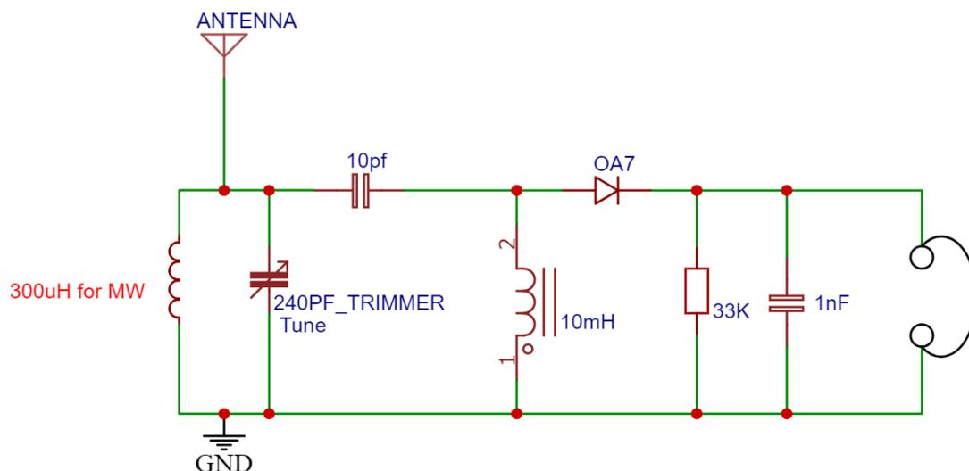
We have now altered the circuit more to allow the antenna to be inductively coupled to the tuning coil to improve the performance from the circuit above. A small two switch will let you change from 'S' for a short antenna, no earth, direct connection to the tuned circuit, or 'L' for long wire with a earth fed to the coupling coil.
