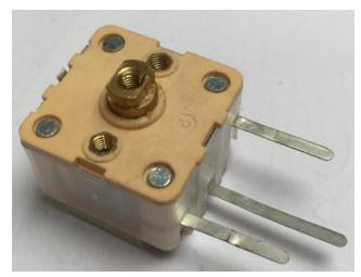
If you have a suitable capacitance meter check between the center pin and the two outer pins, you should find that you have about 270pf when you adjust the capacitor between each pin and center.
