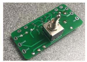
Now turn the board over so we can fit the switch, remove the top nut and washers from the switch and put them on one side for later. The switch should be fitted so its pins **JUST** fit flush with the other side of the PCB, this is so when the ATU is assembled into the case and onto the front plate there is enough of the screws thread protruding to attach the nut to. The nut is only cosmetic really so fitting it really is optional.
