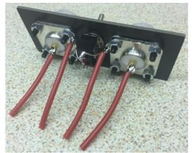
Now fit the links to the back panel, I have provided some silicone coated wire for this, it's very flexible.
