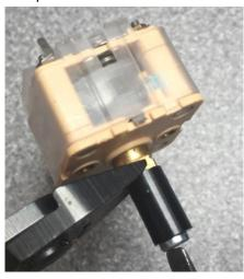
Fold back the three remaining terminals from each capacitor as shown in this picture.
