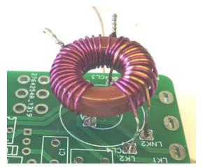
Now fold the 4 wires downwards as per this picture, I find trimming each lead to a different height makes it easier to fit the toroidal to the board, just feed the wires one by one into the correct hole.
