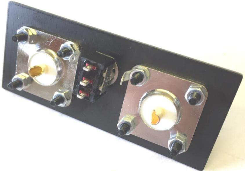
Use the screws/nuts provided to mount the sockets to the back panel. Place the two earth tags on the back of the socket on the holes nearest the switch as per the picture here. If using BNC's tighten the sockets and make sure the earth tag is on the side near the switch.
