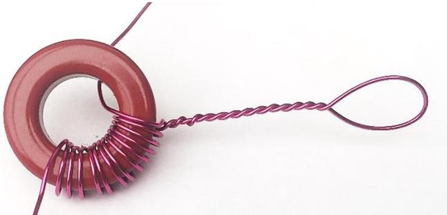
Form a loop about 30-50mm long as shown here, feed the wire back into the core and wind for another 6 turns.
