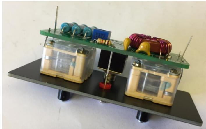
Carefully make sure that the three legs of each capacitor go into their correct mounting holes and that the LED isn't trapped or falls out while doing this. A bit fiddly I know.
