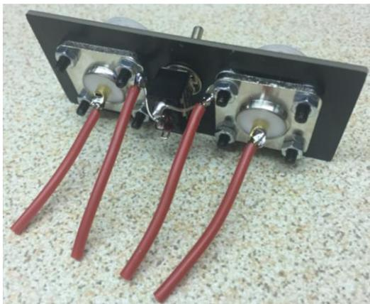
If you have thrown these away then you can also use any sizeable conductor around 1mm<sup>2</sup> or so would be ideal. ( I have also use the offcuts from those 2 watt resistors we fitted earlier, see below)
