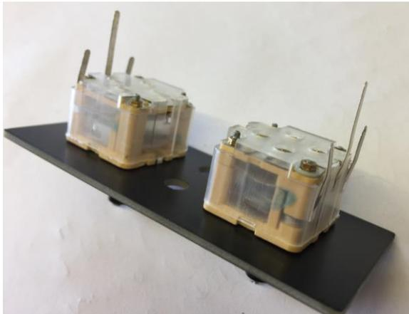
When the capacitors are ready we can move on. Attach the two capacitor to the front plate with the 2.5mm short screws provided.
