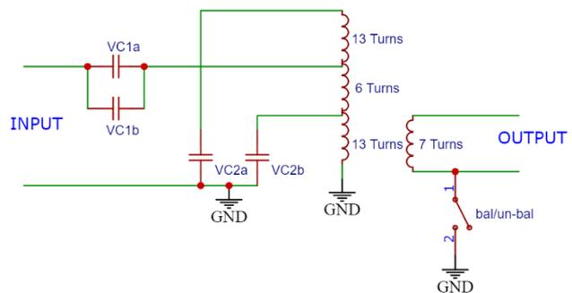
13/6/13 turns on the primary and 7 turns on the secondary, the output can be isolated by means of a grounded toggle switch so the user can use either balance or unbalanced antennas.
