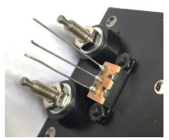
Now back to the front plate, using the off cuts from the other parts already fitted solder 3 straight leads to the contacts on the switch as shown here.
