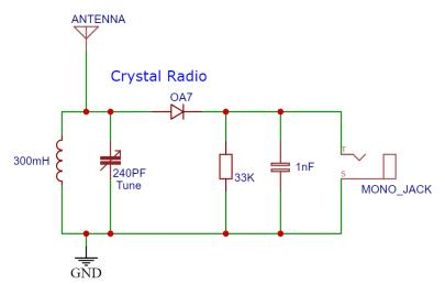
This was a popular circuit that still is used today in many Crystal radio Kits, it does have some problems. With the antenna connected directly to the top of the coil the selectivity is low and the set may only pick up one or two stations, often the same stations can be heard at all points of the tuning control at the same time. This circuit
