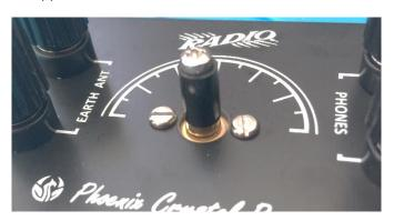
Fit the tuning knob. I just tighten the knob a little at first, just so it grips very slightly, then turn the tuning control and set it so it points correctly. Once you have it set correctly set the control to point upwards and then you can get easy access to the fixing screw, tight then screw to secure the knob.
