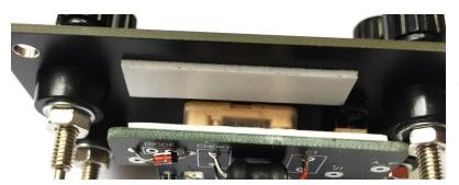
These foam strips help hold the coil in place later.
