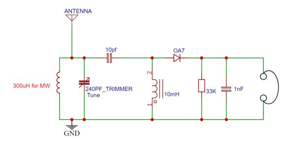
We have now altered the circuit more to allow the antenna to be inductility coupled to the tuning coil to improve the performance from the circuit above.
