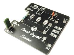
The PCB is designed to make building the crystal radio very easy and trouble free. Larger wide spaced pad have been used so it's suitable for beginners to build (With care!).
