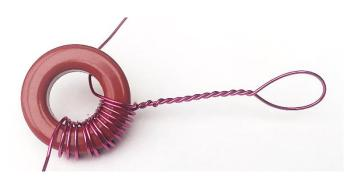
Form a loop about 30-50mm long as shown here, feed the wire back into the core and wind for another 6 turns.
