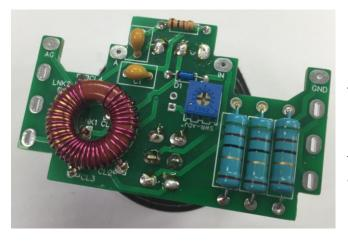
Leave the switches for now and solder all the other board mounting parts (NOT THE LED)
