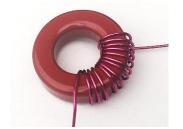
the one end about 50mm long. This counts as one turn, every time the wire passes through the core it counts as a turn,
