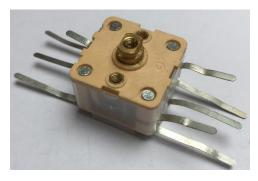
On one side of the capacitor there are 4 pins, the other side has 5. Make sure you identify each side
