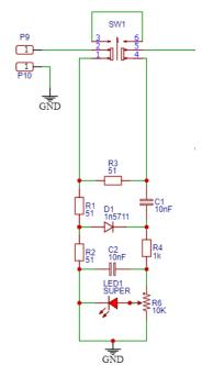
This section can be switched IN or OUT by a two way toggle switch, when in circuit the bridge will light the LED if the antenna is presenting an impedance higher (or Lower) than 50 ohms, if the impedance is matched the LED will go out. Depending on the power level in use the LED can be either too bright and doesn't go out when matched or to dim and hard to see. This circuit has an adjustable sensitive trimmer and it is best to adjust this to suit your most likely used power level.
