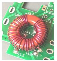
soldering iron for about 10 secs to burn off any enamel on the wire, a fresh blob of solder helps too.
