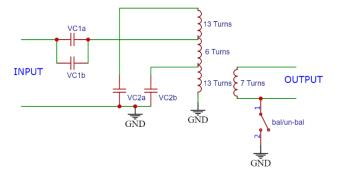
The number of turns on the output stage could be adjusted to work with lower impedance antennas (try just 3 turns if you want to play) the only problem with reconfiguring this setup is that efficiency can suffer
