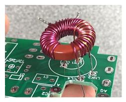
The main winding has 4 connection points, two of which are the loops, we can ignore them for now, the earth side of the winding is nearest the 7 turn coupling coil. The earth side of the winding goes into the pad marked CL4 and the 'hot' end goes into CL1 the coupling coil goes to LNK2 and LNK1.
