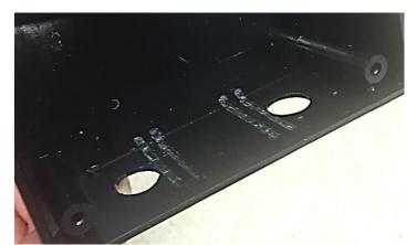
If these guides are not trimmed flush the BNC sockets will not mount correctly. A sharp pair of flush cut wire trimmers do the job quickly and easily.
