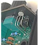
Now we can solder the LED in place. Do not over tighten the pots, we may want to 'jiggle' the front plate when we fit it into the case to get the headphone jack
