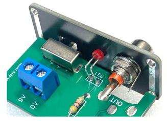
We have a little 3mm LED to fit, that will be the Power On indicator. The LED has two legs and one will be longer than the other. It is very important that the LEDis fitted the right way round. When we have finished mounting the LED the longer leg MUST have been put into the round pads hole.
