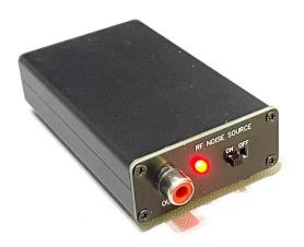
This Kit is designed to help with setting up Receivers filters and audio projects. It will produce strong white noise signals. Starting at audio frequencies right the way into the VHF spectrum. It is not a calibrated test instrument but uses the well know 'Noisy Diode' method of noise production that is amplified by 3 stages to produce a strong signal.
