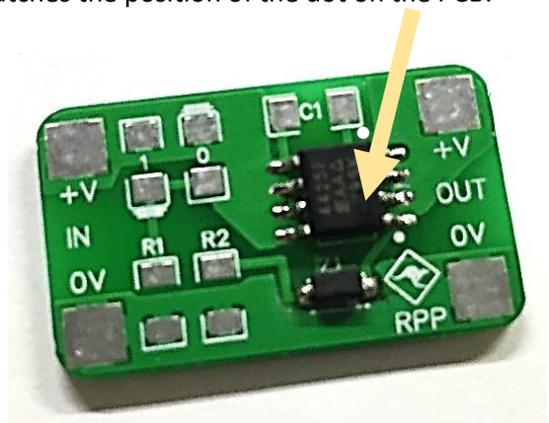
That's the two most difficult parts to fit now done. Double check that the diode and chip are the right way round.
