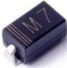
Look carefully and you will see that the diode has a horizontal line at one end. Now this is the difficult part of SMD work I find, the markings can be very difficult to see. You need a good strong light to see the markings. The diode is a Zener diode (Z1) 6v2.
