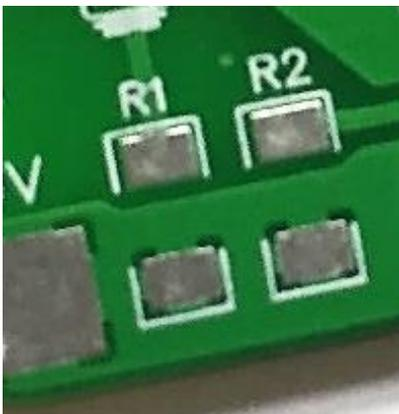
Now we have just two more parts to fit, the resistors R1 and R2.
