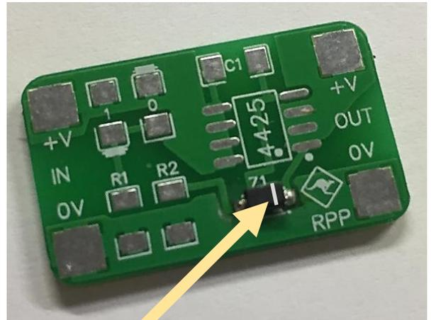
The diode will have a line on one end, this needs to be nearest to the Kanga Symbol on the PCB
