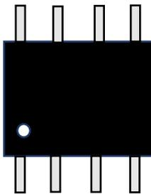
The SI4425 chip must be fitted the correct way round. If you look CAREFULLY you will see a small dot on the top of the chip. This shows where pin 1 is. The PCB shows a small dot near the location of pin1, make sure that the chip is fitted so the dot on the chip matches the position of the dot on the PCB.
