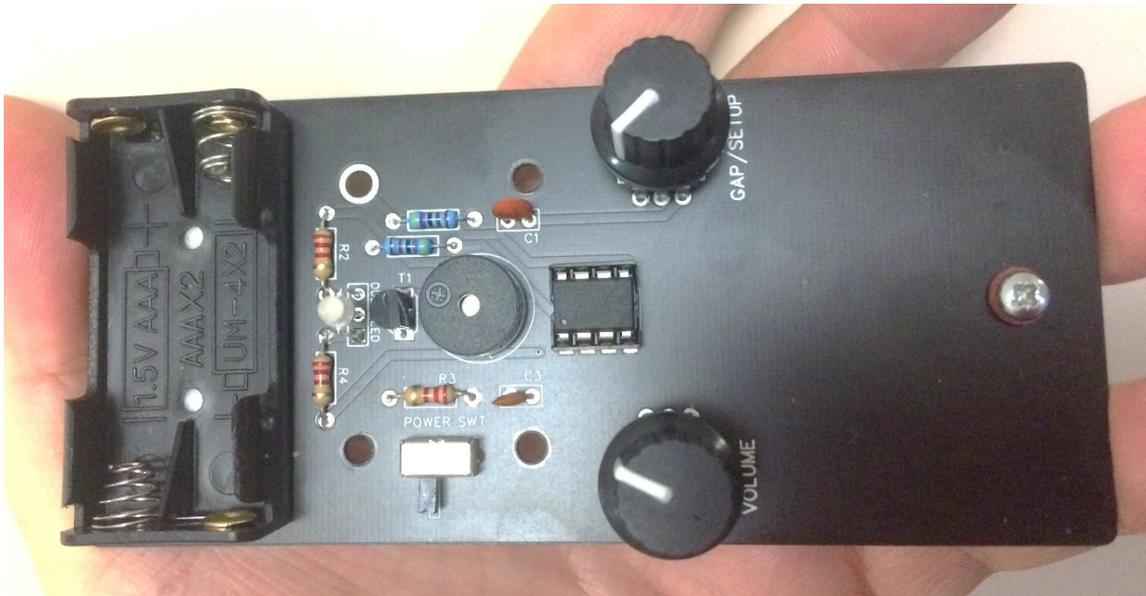
Let's start with the IC socket, make sure you fit it as the layout on the PCB.
