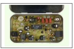
The FOXX-3 by Derek Alexander G4GVM was published in the spring 1999 issue of SPRAT. While based on the original FOXX, it had a few refinements to make operation easier: Automatic transmit/receive change over (semi-break-in), sidetone and built in harmonic filter. Derek has kindly given Kanga Products permission to produce the FOXX-3 in kit form.
