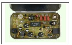
The FOXX-3 by Derek Alexander G4GVM was published in the spring 1999 issue of SPRAT. While based on the original FOXX, it had a few refinements to make operation easier: Automatic transmit/receive change over (semi-break-in), sidetone and built in harmonic filter. Derek kindly gave Kanga Products permission to produce the FOXX-3 in kit form.
