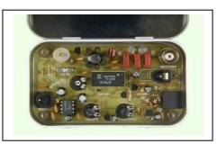
The FOXX-3 by Derek Alexander G4GVM was published in the spring 1999 issue of SPRAT. While based on the original FOXX, it had a few refinements to make operation easier: Automatic transmit/receive change over (semi-break-in), sidetone and built in harmonic filter. Derek kindly gave Kanga Products permission to produce the FOXX-3 in kit form.
