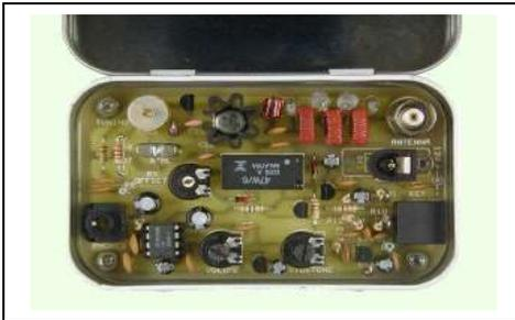
The FOXX-3 by Derek Alexander G4GVM was published in the spring 1999 issue of SPRAT. While based on the original FOXX, it had a few refinements to make operation easier: Automatic transmit/receive change over (semi-break-in), sidetone and built in harmonic filter. Derek has kindly given Kanga Products permission to produce the FOXX-3 in kit form.
