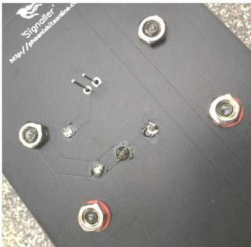
Fix the top panel using the 4 nuts provided, any unused washers can be stored for future use under the front two nuts. That way you will not lose them if you want to change the gap later.
