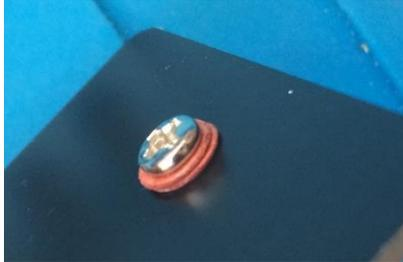
Step One:- Fit the bottom contact screw. Find the 6mm Screw (The shortest in the kit, note yours will maybe a flat slot head) and BEFORE putting it on the bottom board put two of the small Steel washers onto the screw (you may be removing one or adding one later to adjust the gap to your liking). Put the screw through the single hole at the one end of the base panel. The screw head is the bottom key
