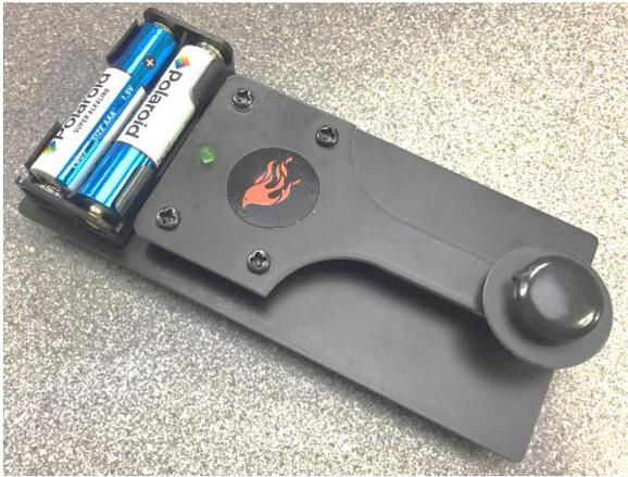
The sticker has not just been included for cosmetic reasons. Try this, hold the key down. Now place your finger tip over the hole in the top of the key panel, you will note that the tone changes. I feel it sounds better with the hole covered, the back pressure blocking the hole just above the sounder changes the pitch and tone qualities. If you agree then place the sticker over the hole.
