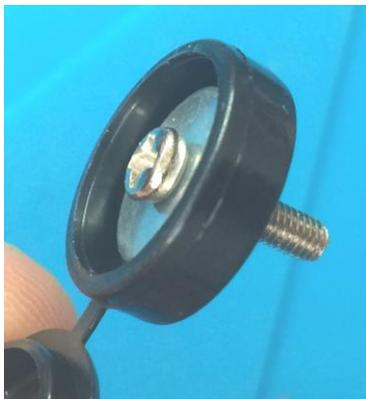
Find the flange, the 3mm white space, one red fibre washer (or steel), the Key top panel and a M3 steel nut.
