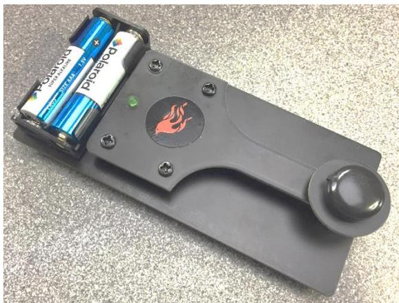
The sticker has not just been included for cosmetic reasons. Try this, hold the key down. Now place your finger tip over the hole in the top of the key panel, you will note that the tone changes. I feel it sounds better with the hole covered, the back pressure blocking the hole just above the sounder changes the pitch and tone qualities. If you agree then place the
