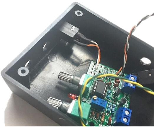
Once you have fitted the key jack then push the PCB in place making sure the LED (and push switch) is seated in their holes, use the washers and nuts provide to secure the board. You will have a little 'jiggle room' to make sure the switch is not trapped against the edge of its hole.
