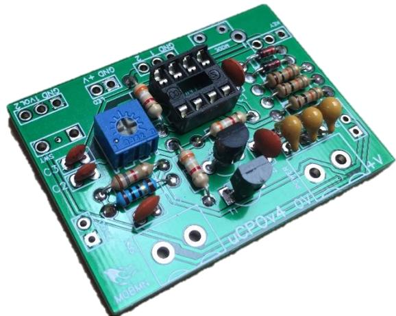
10) Fit the two 2 way blocks, these should be straight forward to fit.
