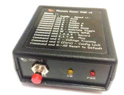
This open source code is now installed on a small but powerful microcontroller. The kit produces a desktop mounting Keyer with many options.
