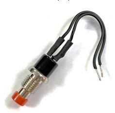
With the kit you will find a short length of wire and some heat shrink. Solder the wire to the two pins of the push button and use the heatshrink to make things nice and tidy, cut the leads to about 50mm.
