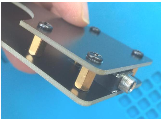
Now drop the top panel onto the base, the black screws should line up with the four fixing holes in the base. Use the four black M3 nuts to attach the two halves. You have two small steel washers left over, these can be used to adjust the gap height. You could easily lose these so I suggest put one under each of the black nuts nearest to the front of the key.
