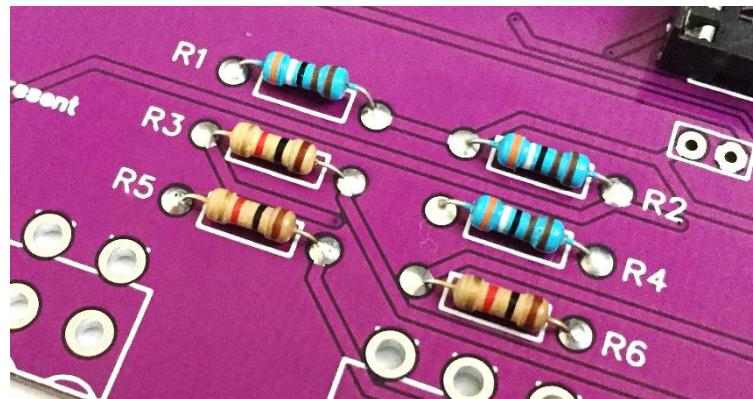
Next fit the 1K Ohm resistors R3, R5, and R6 (first two bands are Brown and Black).
