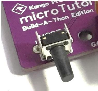
Now we need to fit the Mode selector button, carefully push the pins through the board and make sure the switch is sitting nicely before soldering.
