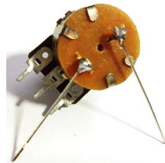
Solder them as shown in the picture below. Use a small piece of heatshrink that came with the kit to insulate one of the wires, no need to shrink this if you don't want to.
