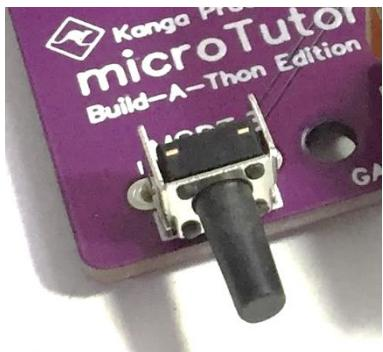
Now we need to fit the Mode selector button, carefully push the pins through the board and make sure the switch is sitting nicely before soldering.
