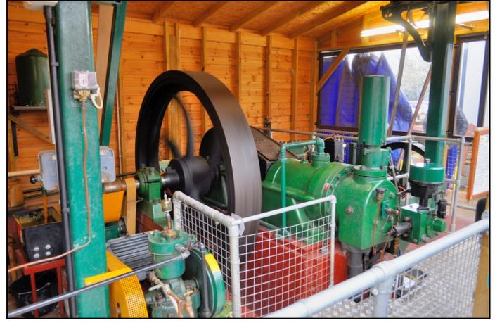
*Outside the main building, the single-cylinder Wilson Oil Engine powered the Massington Lineshaft.*
