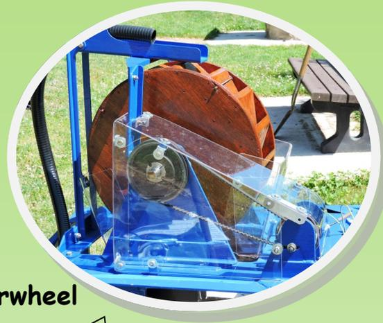
Starting with you pushing and pulling the semi-rotary pump, what is it exactly that makes the waterwheel go round to produce the electricity?
