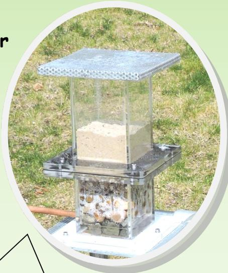
It is the fine sand which filters the water. So what are the pebbles, small stones and large stones underneath the sand for?
